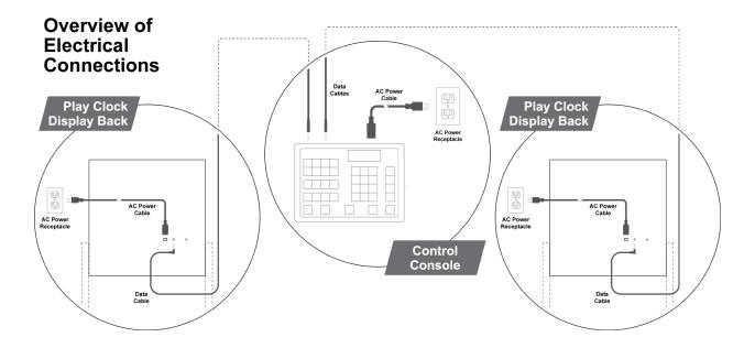
Each play clock cabinet requires a standard power receptacle. If you prefer, you may use a drop cord to bring power to the displays. Electro-Mech provides a detachable power cord with GFCI safety circuitry for each portable display. Plug these cords into the AC power sockets on the backs of the two play clock cabinets. We recommend testing (and resetting) the GFCI feature when you first plug the displays into power receptacles.
