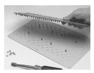
The LED circuit board is held to the mask by several nuts, which you can remove using a 3/8-inch nut driver. On outdoor displays the thick conformal coating can be messy, as the lock washers on the nuts dig into the coating and knock pieces of it away. Be careful to keep the whole assembly right side up when you return it to the play clock cabinet.
