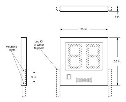
If you wish to attach your play clock displays to a different support structure, you may take advantage of the mounting plates included in the cabinets. These plates have tapped holes, spaced nine inches center-to-center, along the sides of each cabinet. The tapped holes accept 1/2-inch-13 threaded bolts. For Model LX3018, support brackets or posts would need to be positioned 35 inches apart (inside spacing) to provide room for the cabinet.
